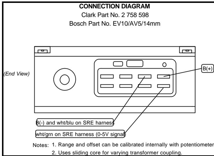
1. Connect the SRE harness to the Bosch throttle as shown in the diagram.
